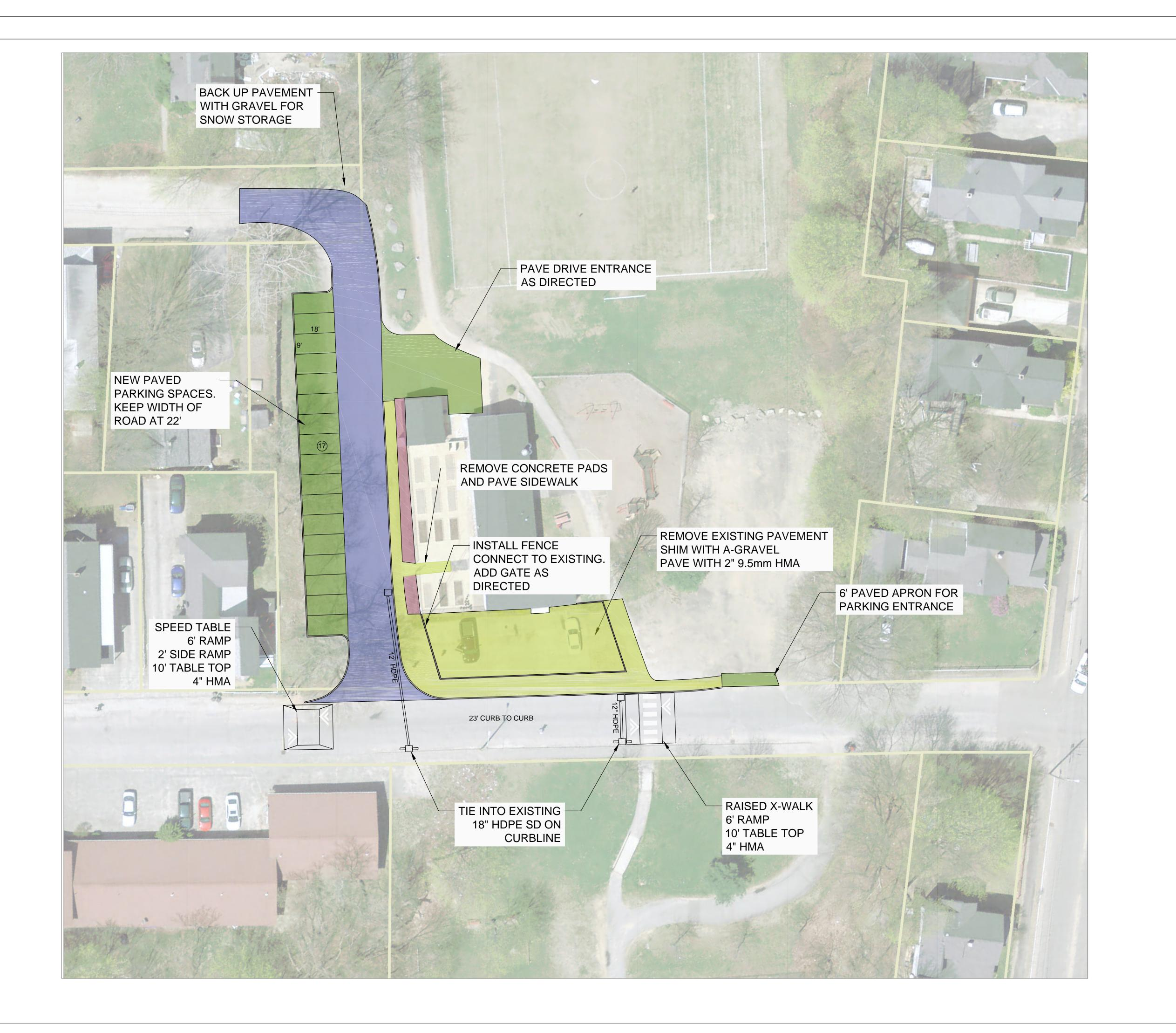
12" - TYPE A GRAVEL 2" - 12.5mm BASE COURSE 1" - 9.5mm SURFACE 2. SIDEWALK BUILDUP 12" - TYPE A GRAVEL 1" - 9.5mm BASE COURSE 1" - 9.5mm SURFACE 3. ROADWAY BUILDUP 15" - TYPE D GRAVEL 3" - TYPE A GRAVEL 2" - 12.5mm HMA BASE 1.5" - 9.5mm HMA SURFACE PARKING BUILDUP SIDEWALK BUILDUP ROADWAY BUILDUP BARK MULCH AREAS Revision/Issue Firm Name and Address Project Name and Address PAL CENTER TRAFFIC CALMING CHESTNUT STREET AUBURN, ME 04210 CHESTNUT STREET CLOSURE 2/1/2019 1" - 20'
